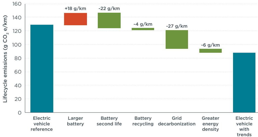
**Figure 3.** Potential changes in battery manufacturing greenhouse gas emissions (compared to reference 2017 electric vehicle) resulting from increased pack size and improvements in battery manufacturing and use.
